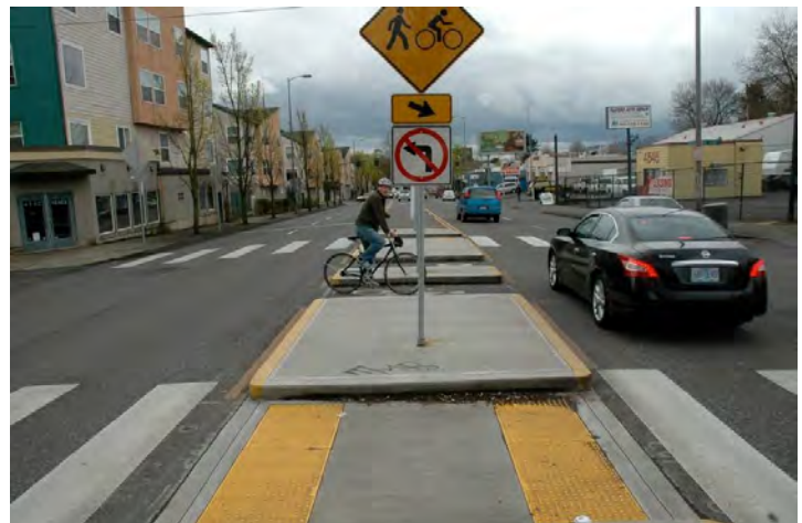
Figure 3.20. Crossing island help reduce stress for bicyclists when crossing intersections. Example in Portland, OR.
